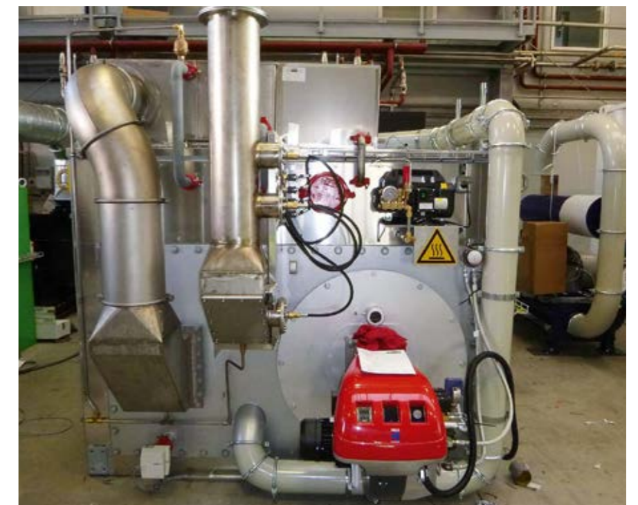
Pre-assembled BOOSTER for installation inside a building
